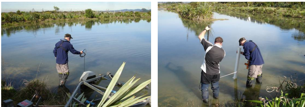
Figure 3: Dudley Bell measuring conductivity (on left) and Dudley Bell and Warrick Powrie measuring black disc water visibility (on right). Photo: Eddie Sides.
